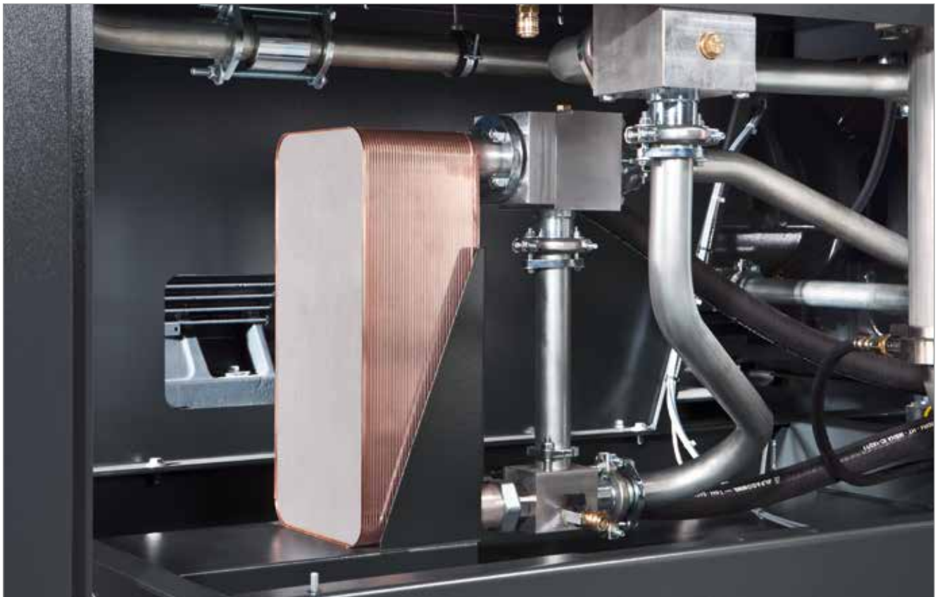
Image: Internal layout of a compressor – system comprising plate-type heat exchanger, thermostatic valve and complete pipework
